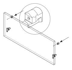
**3** Connect the left and right profiles to the steel back panel.
