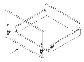
6 Connect the steel back panel to the front panel using the lengthwise railings (left + right).
