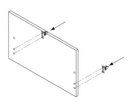
Attach the railing fixing with 2 truss head screws M3x10.
