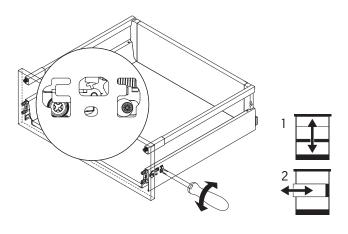
11 Adjust the angle of the front panel on the lengthwise railing. Then slide the cover cap forward.
