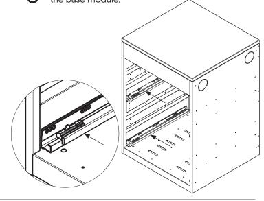
9 Slide the drawer onto the cabinet profiles in the base module.
