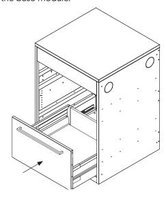
10 Adjust the front panel in height and at the sides in order to get an even gap.
